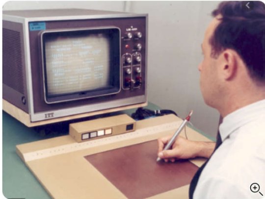
1964, The RAND Tablet: A Machine Graphical Communication Device.
